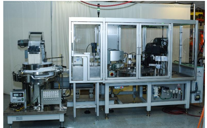
Automated line, based on a rotary table, for a medical diagnostic product. Courtesy of CAID Automation
