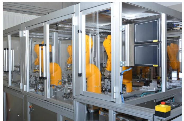
Fully automatic line with 8 robots for a medical device. Courtesy of CAID Automation
