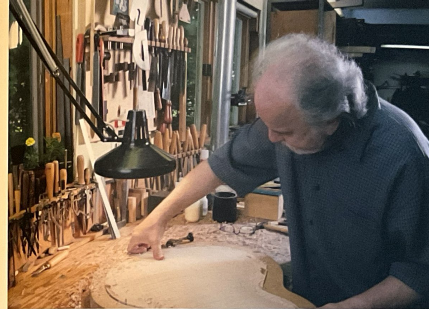
Testing the flexibility of a carved back requires the skill to create the proper arch, the knowledge to know when optimum thickness is reached and a strong thumb.
