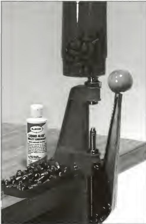
Figure 49 Lee Sizer mounted on a Reloader press.
