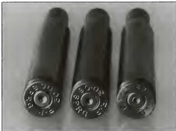
Figure 43 Primer 1 is a light load. Number 2 is a normal NEVER EXCEED load. Number 3 is a hot load. Can you see the difference?
