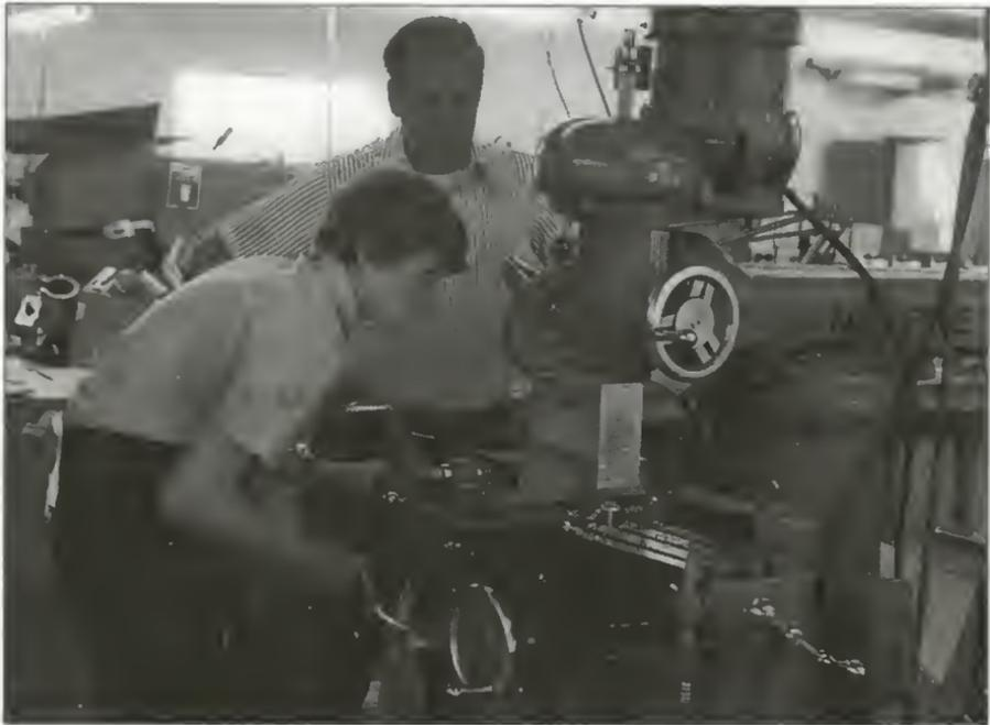
*Figure 8 The picture is my son John in 1975 starting the first prototype press. That solid chunk of aluminum was converted into the attractive turret press in the next picture. You can see the influence the All American had on my thinking. The finished press worked well, but was no better than the All American. The design was discarded. John was 16 at the time. He had already worked with me for two years. Photo is by Dean Grennell on one of his visits to our plant in Hartford.*
