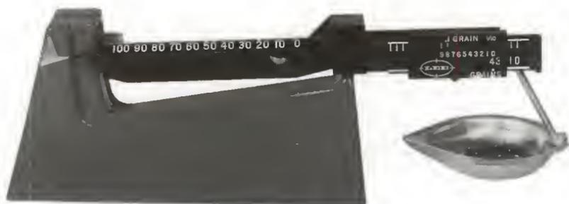
Figure 39 Lee Safety Scale for measuring gunpowder.
