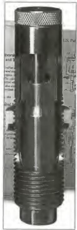
Figure 24 Cutaway of The Lee Collet Die
