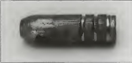
Figure 40 Cast bullet shows rifling stripped.
