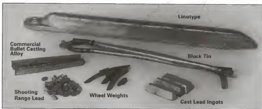
Figure 45 The stuff bullets are made from.
