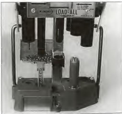
**NOTE** The 8 segment crimp starter is in the front on the 12 GAUGE only. the other gauges have the 6 segment starter in the front. Be sure you select the correct one.
