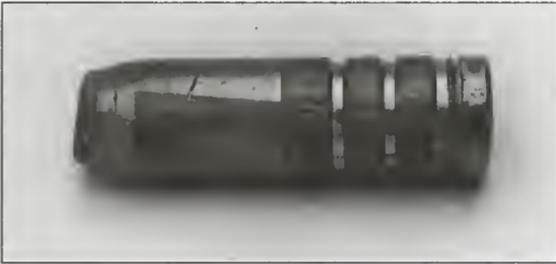
Figure 41 Rifling in good condition at higher velocity.
