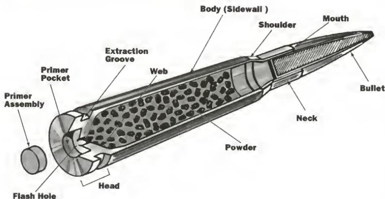
*Figure 1 Cutaway of a Typical Rifle Cartridge.*
