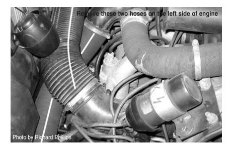
know you had. I found that the opening through which you reach the plugs is nearly exactly the depth of my spark plug socket and a 3" extension, so the socket wrench wouldn't quite fit well enough to actually get a grip. A 6" extension is way too long to fit, so the solution is to pick up a 1" "wobble" extension. The "wobble" feature comes in handy as you'll find that the skill of contortionism to be a requirement.
