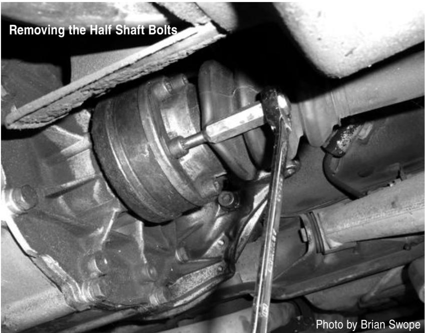
**Removing the Half Shaft Bolts**
