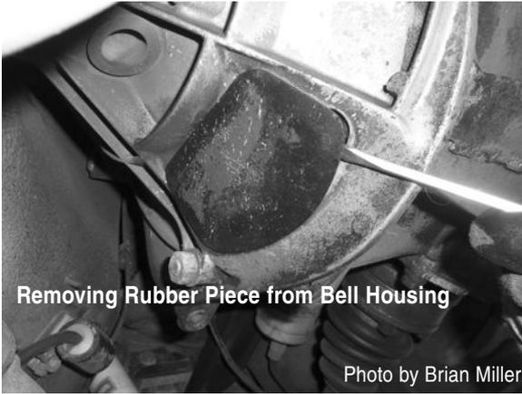
**Removing Rubber Piece from Bell Housing**
