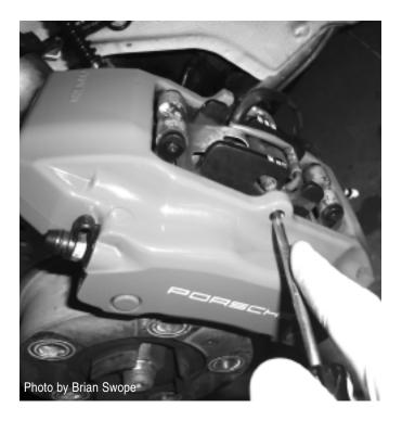
6. Add a bit of grease to the inside flat piece of metal. This is a squeal deterrent.
