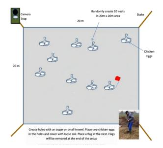
The diagram above provides you with an overview of how to set up the survey on site. The small double white circles that you find in the grey box represent the store bought chicken eggs and the holes in the ground.
