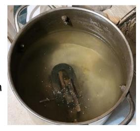
the mold keeping the torch on it at all times. I spilled silver on some of the pours and had to have Dick pour some for me. Then I quenched it and took it out of the mold.
