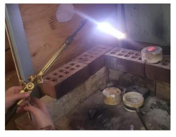
Next, I annealed the planchets to make them softer for stamping. I used the torch again. First, I heated an upside-down crucible then put the planchet on it and carefully heated
