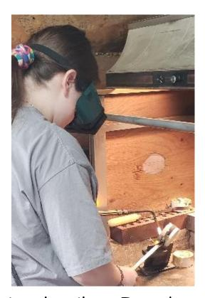
tokens). The first step was melting the silver. I used a propane oxygen torch. I first heated the crucible to glowing. Then I melted one ounce of silver to molten and added another ounce.
