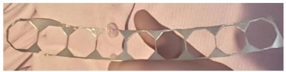
same size holes from my planchets. Then I set the thicker plug on the hole of the planchet in between two dies under the screw press. I whacked it with the screw press to push it into the hole. Sometimes it even snapped in. The plugs raised the planchet's
