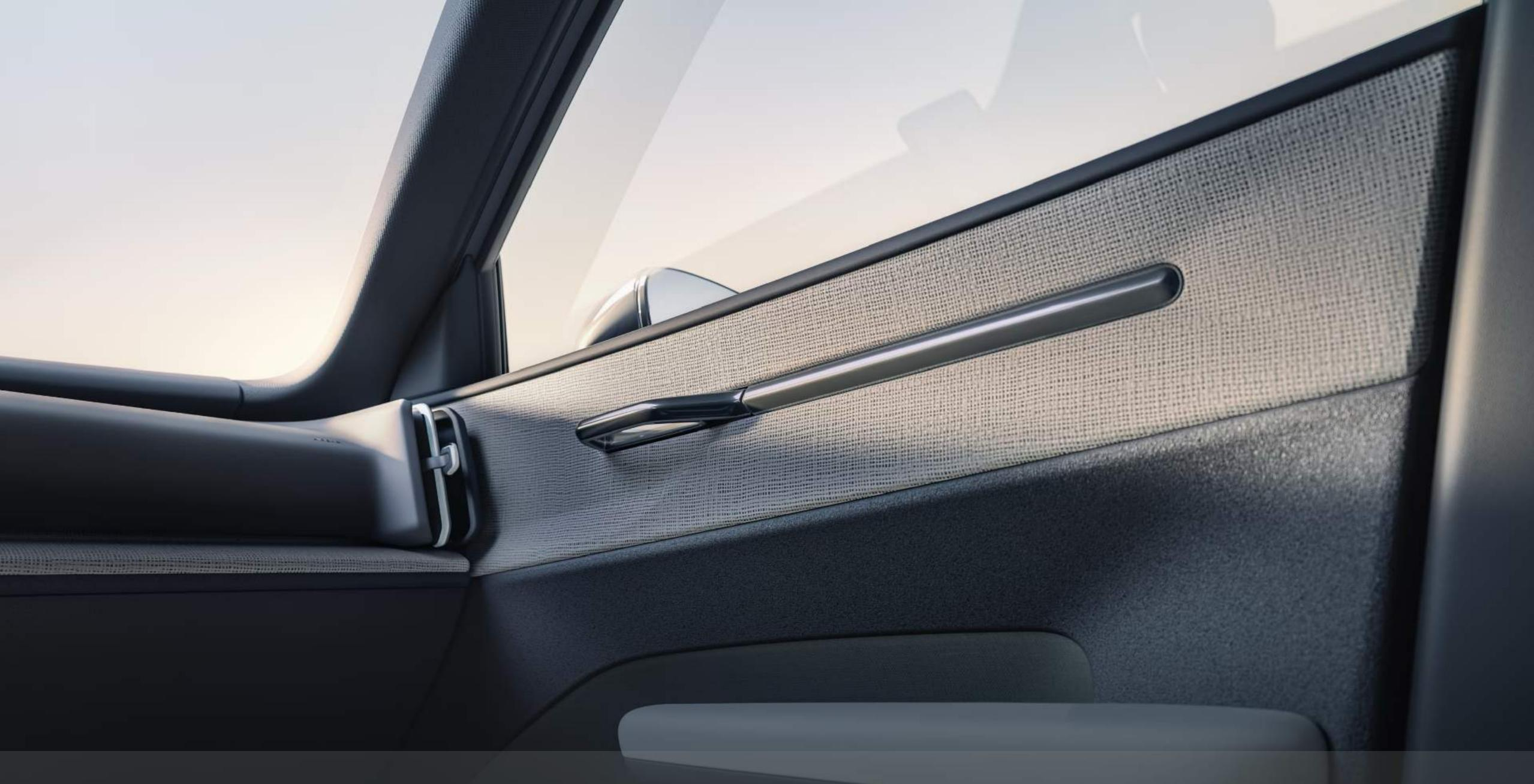
Developed to complement bio-attributed and recycled synthetic surfaces, the interior material palette ensures seamless integration of sustainable elements. Composed of recycled PET and bio-based polymers, these surfaces enhance both environmental responsibility and material longevity.
