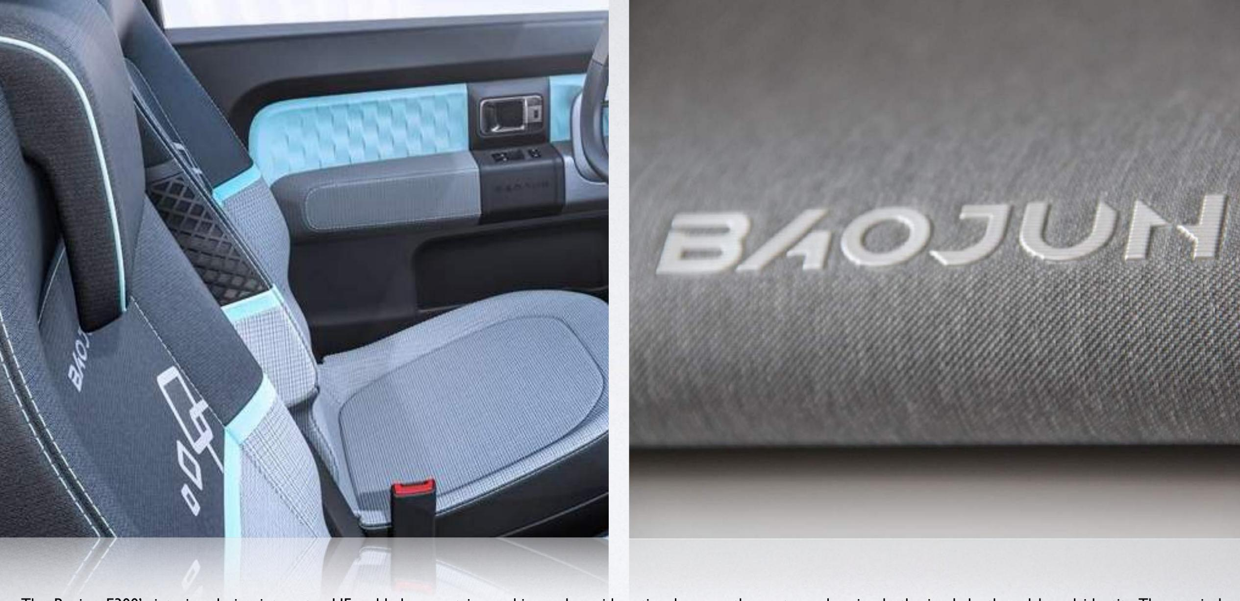
The Baojun E300's interior design integrates HF-welded geometric graphics and a mid-section logo on the seats, enhancing both visual depth and brand identity. The precisely embossed patterns complement the melange fabric's natural texture, creating a layered interplay of material and form. This fusion of structured detailing with soft textiles reinforces the vehicle's modern, tech-inspired character while maintaining a cohesive interior aesthetic.
