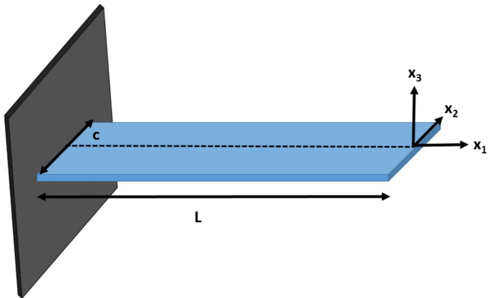
Figure 1: Thin cantilevered Kirchhoff plate which will deform according to aerodynamic lifting forces.
