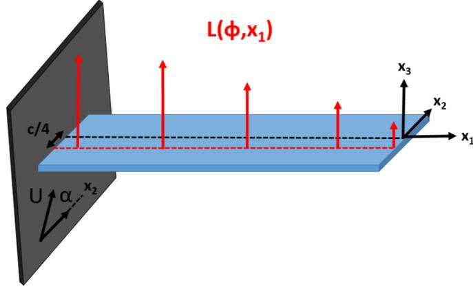
Figure 2: Lift forces are fixed at the quarter chord point for the flow of velocity  $U$  making an angle  $\alpha$  up from the  $x_2$  axis. The lift force varies with the span position  $x_1$  and the angle of rotation of the elastic plate, making this problem non-linear in the applied loads.
