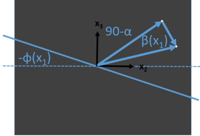
Figure 3: Cross-section of deformed plate with freestream velocity at angle  $\alpha$  to  $x_2$  axis, correction angle  $\beta$  from downwash velocity, and elastic rotation  $\phi$ .
