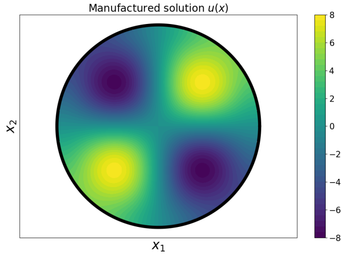
Figure 4: The assumed temperature field used in the method of manufactured solutions, from which the source term and inhomogeneous Dirichlet BCs are computed.
