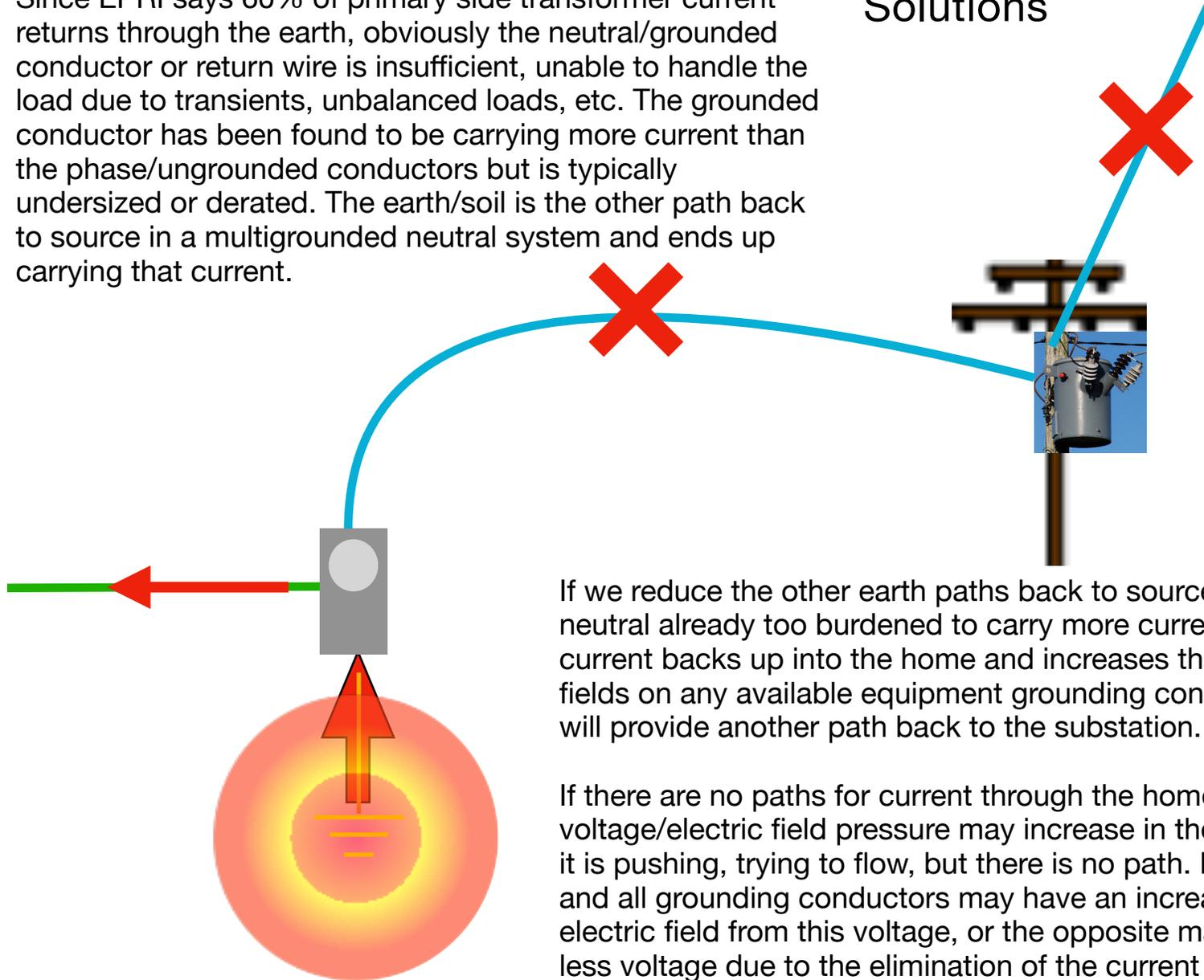
If we reduce the other earth paths back to source, with the neutral already too burdened to carry more current, the current backs up into the home and increases the magnetic fields on any available equipment grounding conductor that will provide another path back to the substation.
