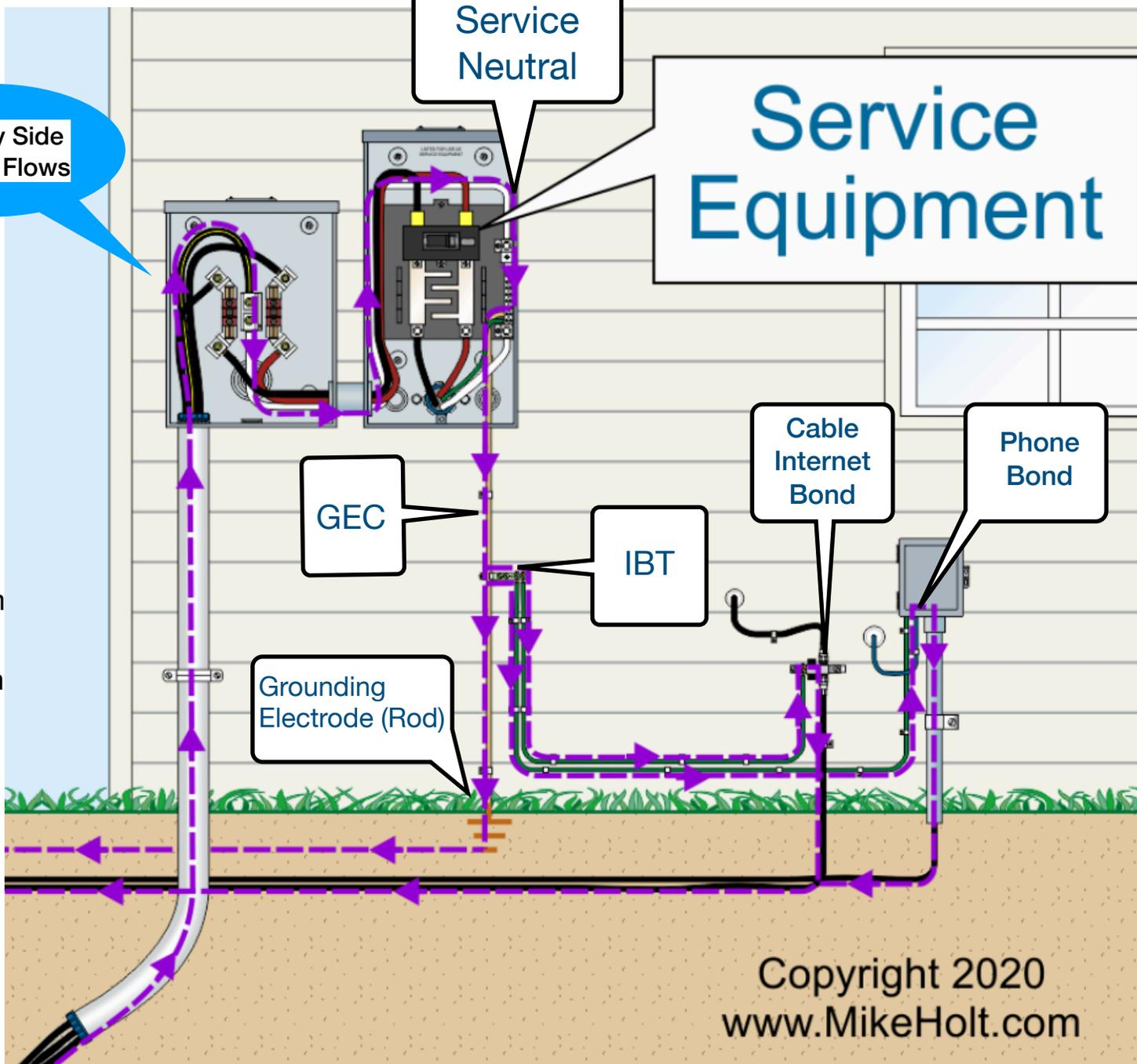
Primary Return Current is both through the earth and the wires/conductors, especially the Service Neutral which connects to Equipment Grounding Conductors associated with any metallic appliance making an electrically conductive connection to earth.
