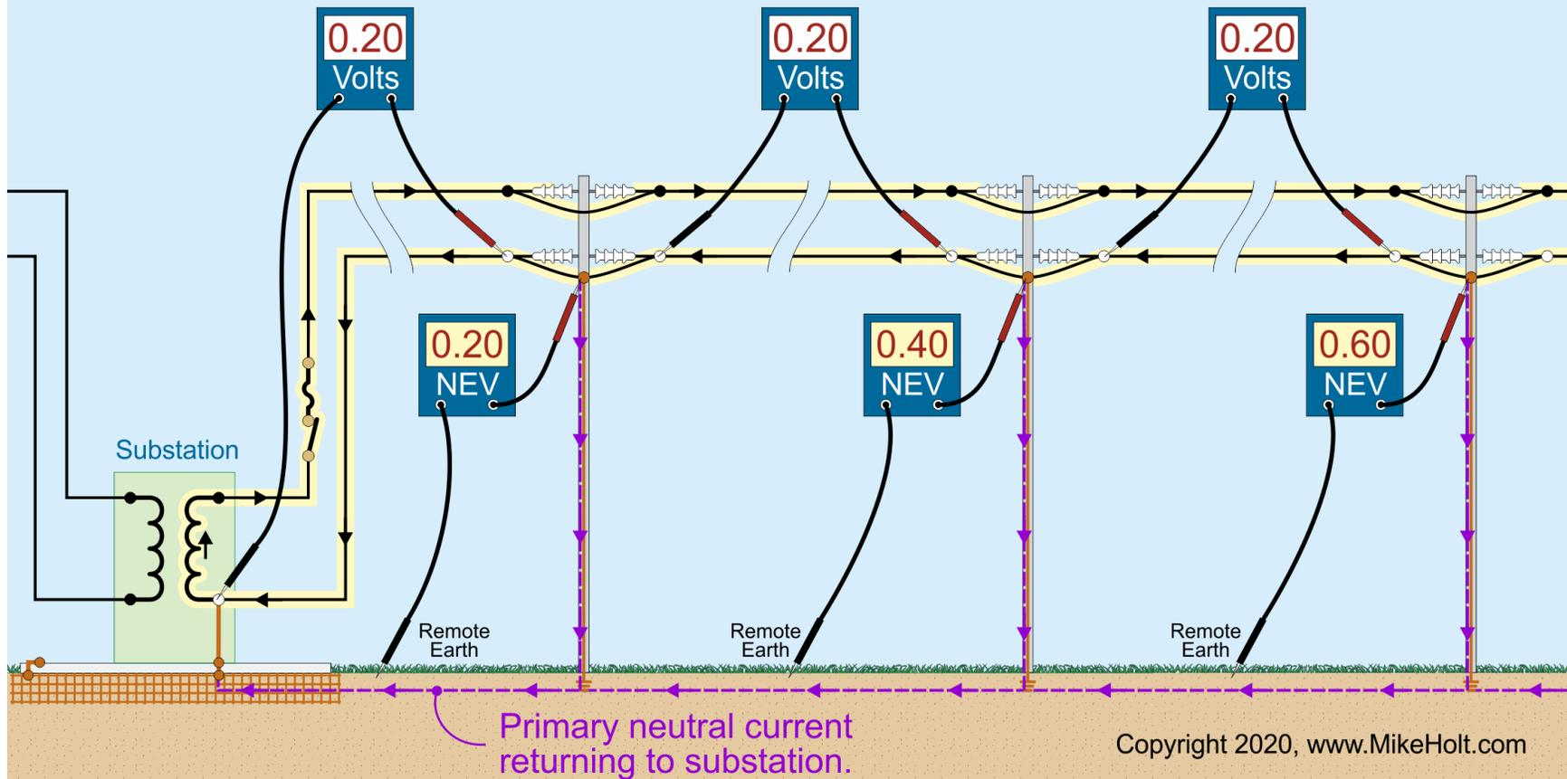
The voltage drop of the primary neutral conductor is dependant on the impedance of the neutral return path and the magnitude of the return current;  $E = I \times R$ .
