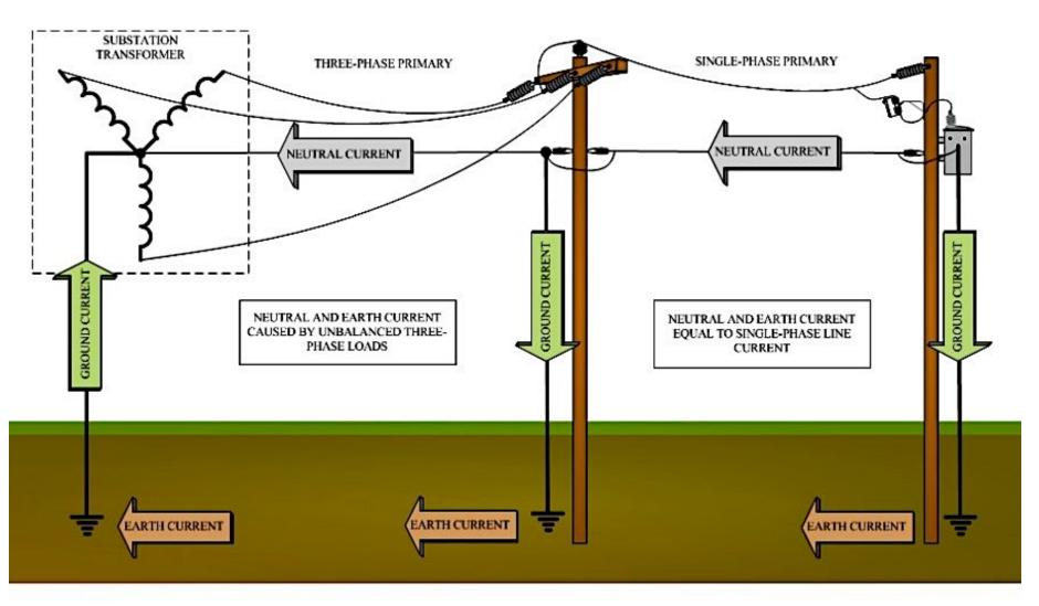
Figure 16—Normal neutral, ground and earth current paths in a multi-grounded Wye distribution system
