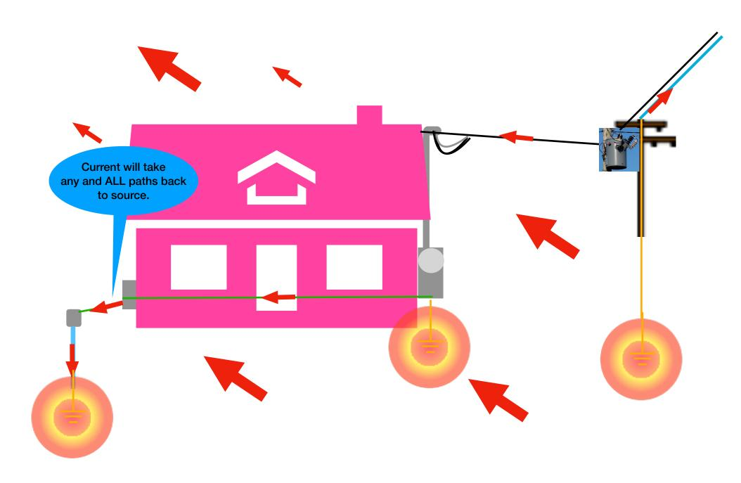
50 mA, split into two paths of equal resistance/ impedance, will end up having 25 mA on each path.
