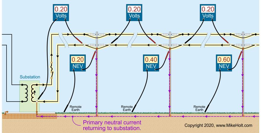
The voltage drop of the primary neutral conductor is dependant on the impedance of the neutral return path and the magnitude of the return current;  $E = I \times R$ .
