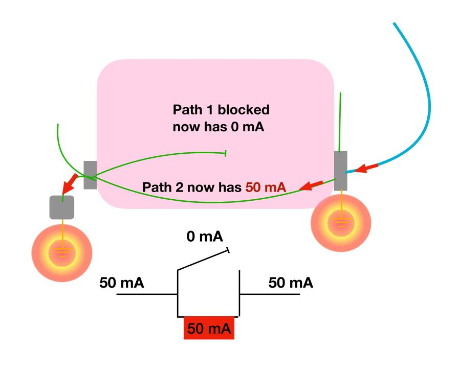
When you reduce the number of paths, Magnetic fields will be INCREASED around the remaining wires carrying the "foreign" current.
