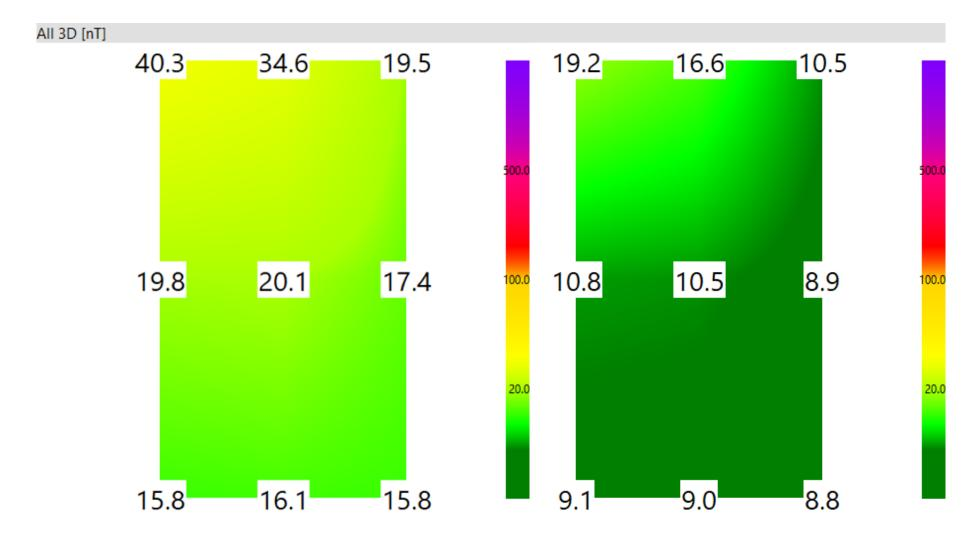
(H.A.), head of bed, Heat/Furnace power on (left side picture), then off (right side picture)
