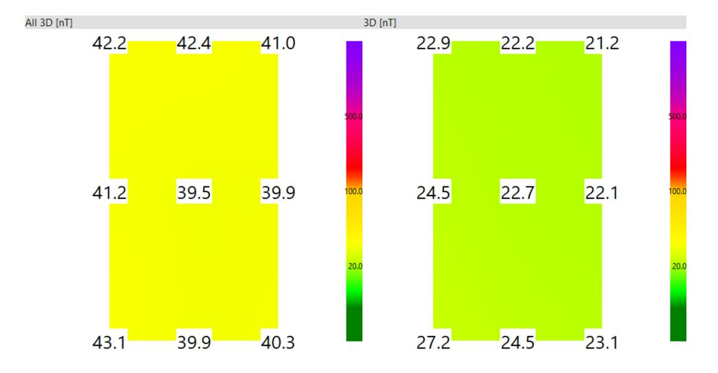
(J.S.) Upstairs bedroom localized magnetic field from coolant line bundle (left side picture). Power off to Furnace removed magnetic field (right side).
