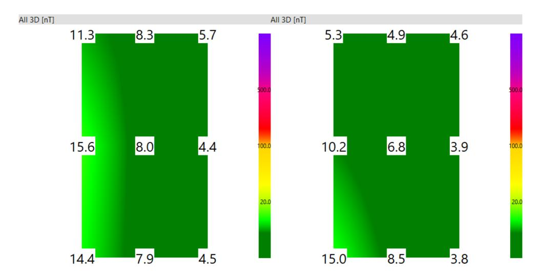
(M.B.) Left side before ground loop isolator installed on cable line. Right side, after ground loop isolator installed.
