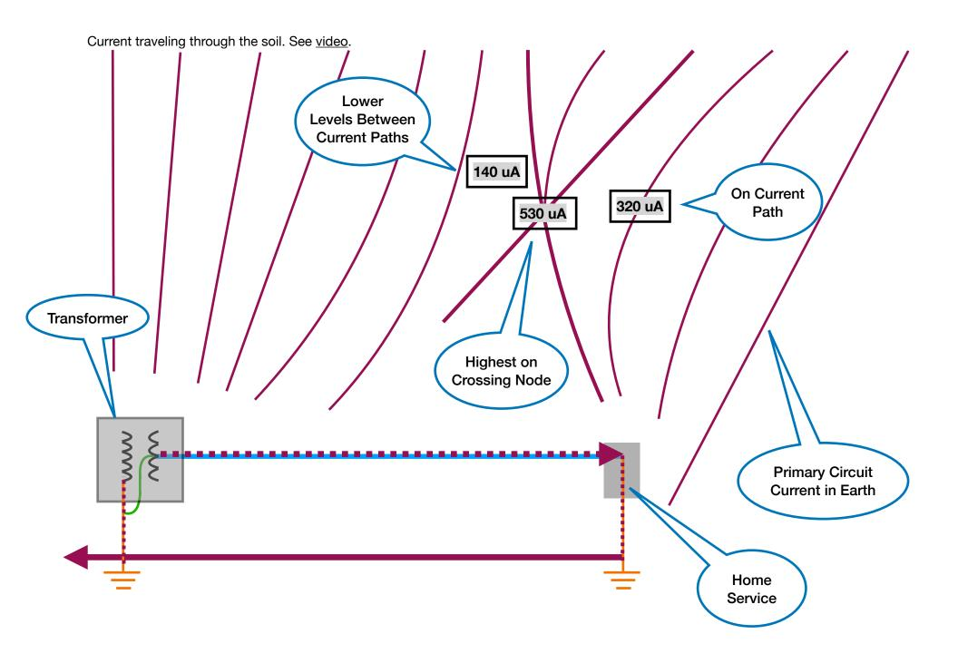
Only one current flow path is shown here (red arrows) but imagine how many there can be making loops between appliances, on the water and gas pipes, and especially on anything that connects back to the earth. Not shown are all the paths throughout the equipment grounding conductor system in branch circuit outlets and lighting systems. These all create magnetic fields in the home and higher contact current conditions.
