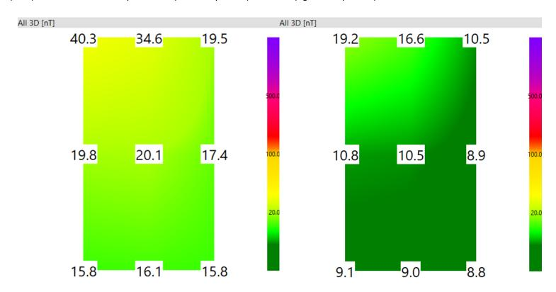
Case 2 (J.S.), head of bed, Heat/furnace power on (left side picture), then power off (right side picture).
