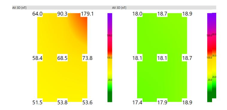
Case 3 (T.A.) Before NCB installed on Furnace (left side). Then after installed (right side).
