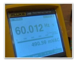
If you have power on in the room, there is still 60 Hz electric fields all around you and the Fluke 287 will be recording that energy upon your body and on the grounding conductor. Turning off the power, greatly reduces that 60 Hz power and the remaining frequencies are much easier to address and manage.
