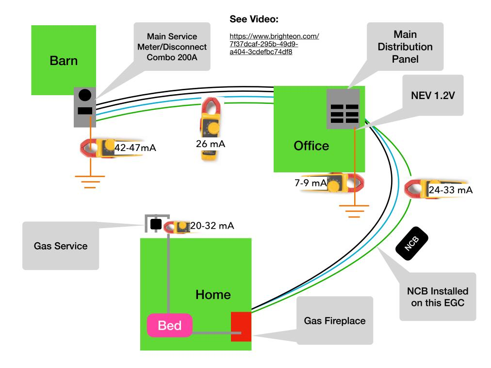
33 mA on EITHER the Neutral or EGC feed when connected to **Home Circuit EGC** 33 mA Office **Home Branch Circuit** EGC attached to Gas Fireplace and pipe
