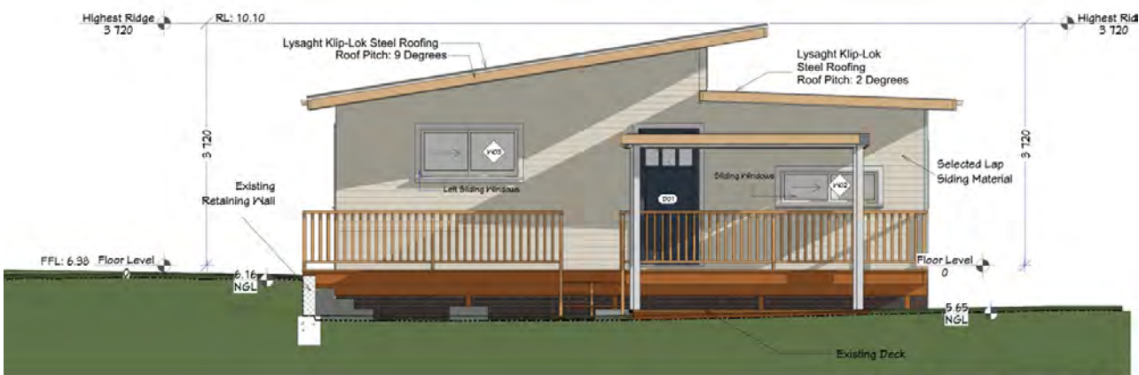
East Elevation (E1)
