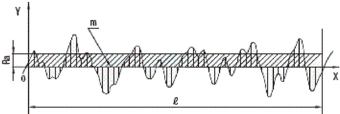
**Figure 1.** Measurement of  $R_a$
