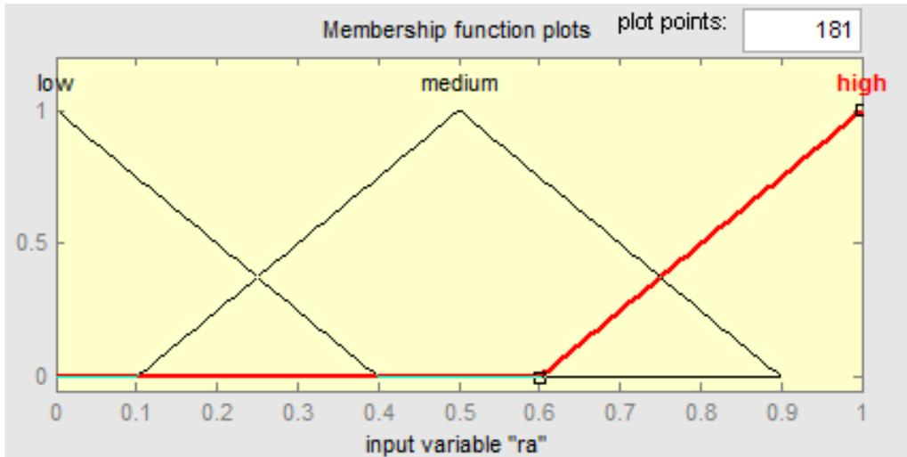
**Figure 6.** Membership functions (MFs) for Ra (normalized SN ratio of Ra)
