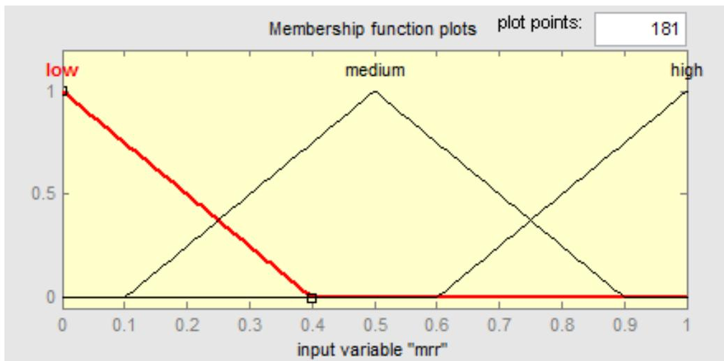
**Figure 5.** Membership functions (MFs) for MRR (normalized SN ratio of MRR)
