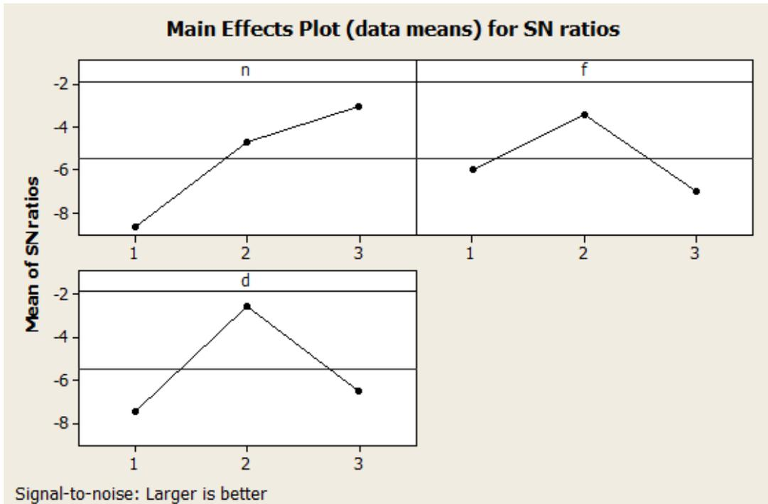
**Figure 9.** Evaluation of optimal setting (SN ratio plot of MPCIs)
