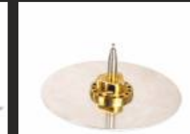
measuring system for plaster mix
