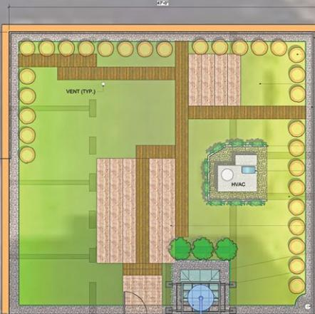
EXISTING DOOR TO GREEN ROOF AREA. 1 STEP DOWN TO TO RAMP LANDING, THEN 2 STEPS DOWN TO DECKING (4 RISERS). DOOR THRESHOLD IS 24" ABOVE DECKING. LANDING IS 18.25' ABOVE DECKING.
