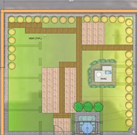
EXISTING DOOR TO GREEN ROOF AREA. 1 STEP DOWN TO TO RAMP LANDING, THEN 2 STEPS DOWN TO DECKING (4 RISERS). DOOR THRESHOLD IS 24.5' ABOVE DECKING. LANDING IS 19.25' ABOVE DECKING.
