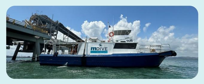
The Gun is a modern design utility vessel of a single chine planning hull configuration. Construction is in heavy duty welded marine grade aluminium with welded aluminium superstructure, incorporating a fly bridge driving station.
