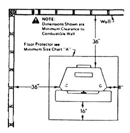
FIGURE 3 WALL INSTALLATION
