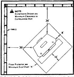
FIGURE 4 CORNER INSTALLATION
