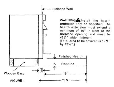
Base for BUCKMATE must be level with or slightly higher than finished hearth height - dimension (A) Figure 1. Front of BUCKMATE cabinet must be recessed 2½" from finished wall.
