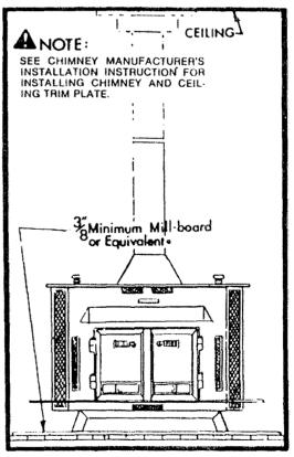
FIGURE 7 CHIMNEY MOUNTING
