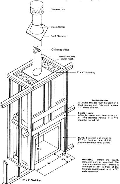
FIGURE 3 EXTERIOR ROOF OR CHASE
