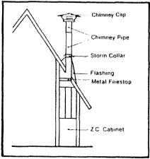
FIGURE 2 Through High Pitch Roof
