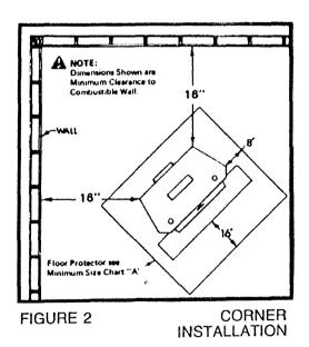
CAUTION: There must be a minimum of 18" from any single wall pipe to a combustible wall. If there is not 18" from single wall pipe to the combustible wall, a wall protector must be used.
