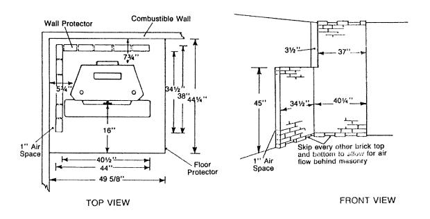
3. Using 24 ga. sheet metal with 1" ventilated air space.
