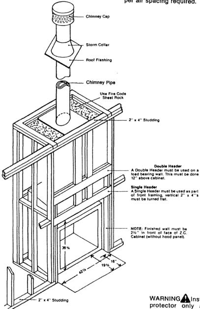
FIGURE 3 EXTERIOR ROOF OR CHASE
