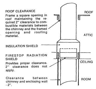
8" Chimney fits between standard 16" OC joists.
