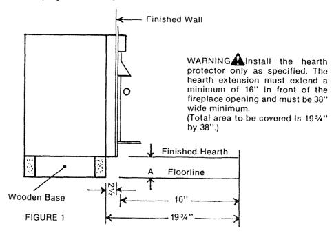
Base for BUCKMATE must be level with or slightly higher than finished hearth height - dimension (A) Figure 1. Front of BUCKMATE cabinet must be recessed 2½" from finished wall.
