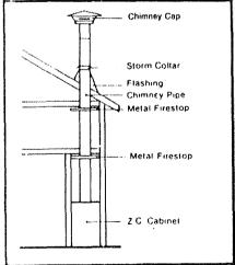
FIGURE 1 Through Ceiling & Normal Pitch Roof
