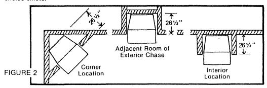
Above (Figure 2) are framing location examples with depth dimensions for some typical configurations. These are finished measurements so install accordingly.
