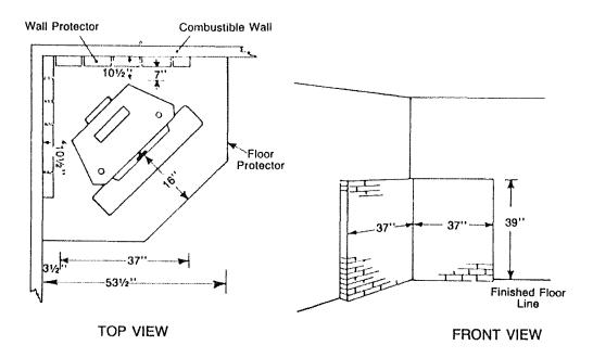
2. Using 31/2" masonry with 1" ventilated air space.
