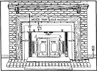
FIGURE 8 INSTALLED MINIMUM CLEARANCES
