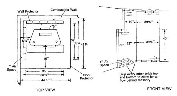
3. Using 24 ga. sheet metal with 1" ventilated air space.
