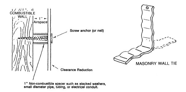
Masonry walls may be attached to combustible walls using wall ties.
