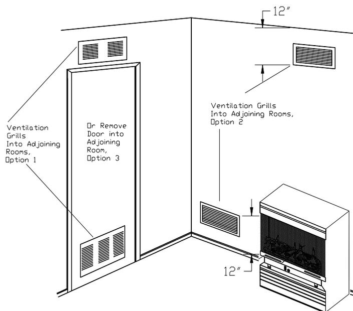
Figure 7: Ventilation Air From Inside Building
