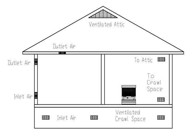
Figure 8: Ventilation Air From Outdoors
