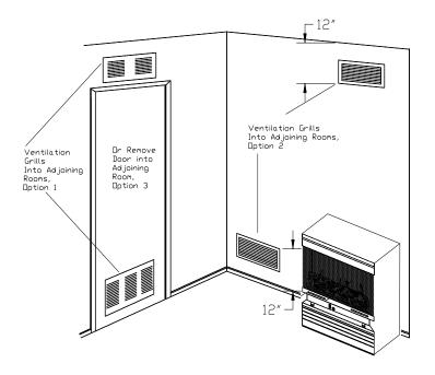
Figure 7: Ventilation Air From Inside Building **NOTE:** Drill holes on bottom of pedestal base on each corner. Unit must be fastened to floor with screws.
