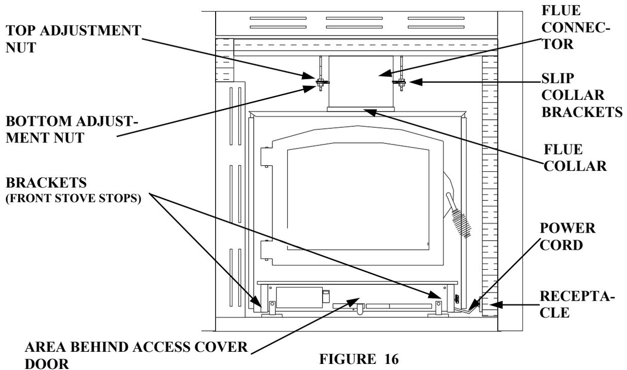
4. Remove the access cover door located at the bottom front of the room heater. There are two (2) philips head screws which must be removed, one (1) in each top corner of the access cover door.
