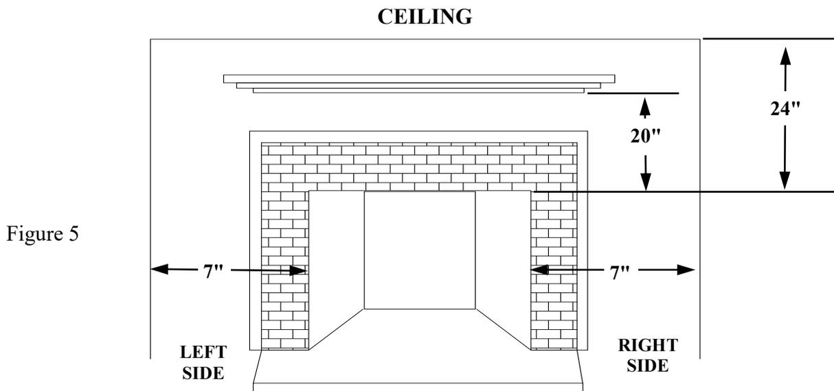
**NOTE:** If used in installation trim panels or surrounds shall not seal ventilation openings in fireplace. Also provide adequate clearances around air openings
