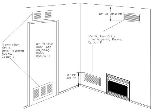
Figure 13 Ventilation Air From Inside Building
