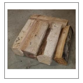
Run 2 – Test Fuel Loaded into Stove
