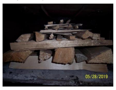
Open the by-pass and use a torch for 40 seconds to one minute to ignite the fuel, focusing the torch on the top middle portion of the load. Leave the door open around two inches for 1.5 to 2.5 minutes. After three to four minutes, close the by-pass. The amount of time for both the door and the by-pass are to be based on how involved the fuel is.
