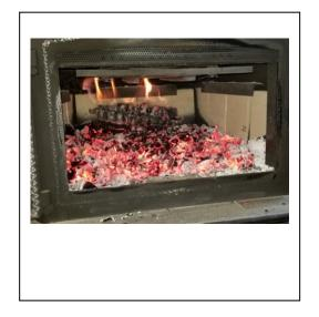
**Run 4 – Test Fuel Loaded into Stove**
