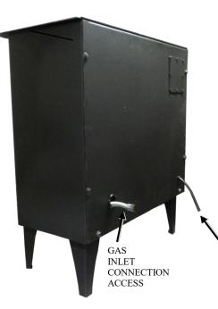
Installation must include an equipment shutoff valve, union and plugged 1/8" NPT tap. Locate NPT tap within reach for test gauge hook up. NPT tap must be upstream from heater (See Figure 8).
