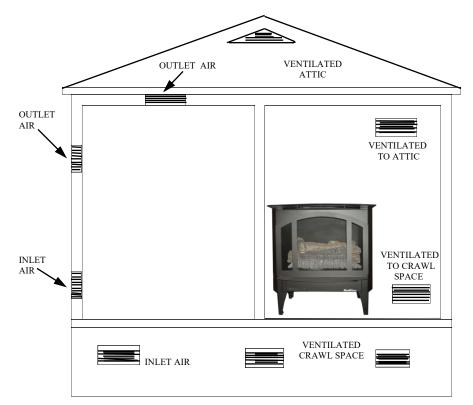
FIGURE 3 - VENTILATION AIR FROM OUTDOORS
