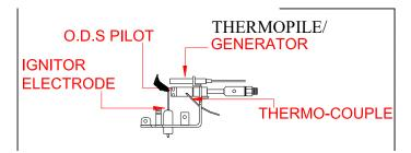
FIGURE 19 - INCORRECT PILOT FLAME PATTERN L.P. OR NAT. GAS
