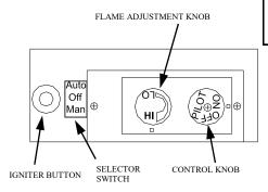
FIGURE 16 - CONTROL KNOB AND IGNITER BUTTON LOCATION \*If knob does not pop up when released, stop and immediately call your service technician or gas supplier. \* If the pilot will not stay lit after several tries, turn the gas control knob to the "OFF" position and call your service technician or gas supplier.
