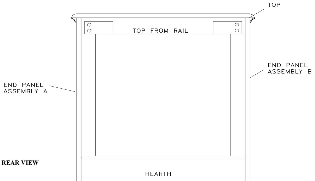
After assembling the WS you must insert the ZCBB. It is best to insert ZCBB from rear of WS, this gives you more area to hold ZCBB and reduces risk of scratching surface of the base (hearth) area. Flush and center ZCBB's front in the WS.
