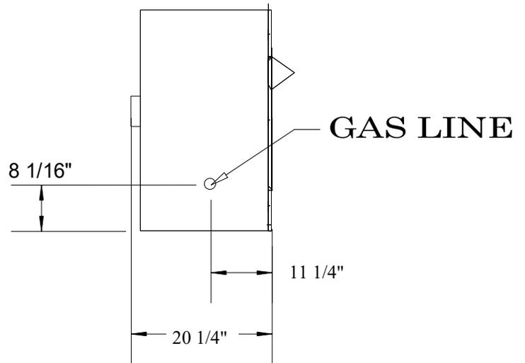
**WARNING: INSULATION OR OTHER MATERIALS MUST NOT BE PLACED AROUND OR NEAR THE FIREBOX. FILLING THE SPACES AROUND THE FIREBOX CAN CAUSE A FIRE OR RESULT IN PROPERTY DAMAGE, PERSONAL INJURY OR LOSS OF LIFE .**
