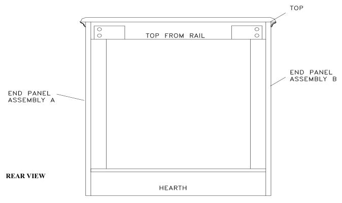
After assembling the WS you must insert the ZCBB. It is best to insert ZCBB from rear of WS, this gives you more area to hold ZCBB and reduces risk of scratching surface of the base (hearth) area. Flush and center ZCBB's front in the WS.
