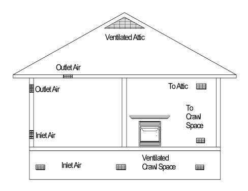
Figure 7 Ventilation Air From Outdoors
