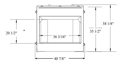
WARNING: NOTCHING OF FRAM-ING AROUND THE STANDOFFS (SPACERS) OR ALTERATION OF THE STANDOFFS CAN CAUSE A FIRE OR MAY RESULT IN PROP-ERTY DAMAGE, PERSONAL IN-JURY OR LOSS OF LIFE.
