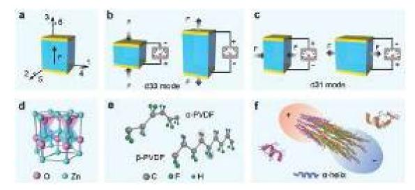
Fig. 2 Piezoelectric materials and piezoelectricity. (a) Direction of forces affecting a piezoelectric element. Illustration of the  $d_{33}$  (b) and  $d_{31}$  (c) working modes. (d) Wurtzite-structure model of inorganic piezoelectric material ZnO. (e) The  $\alpha$ - and  $\beta$ -phase structure of organic piezoelectric polymer PVDF. (f) Natural piezoelectric material of M13 bacteriophage.
