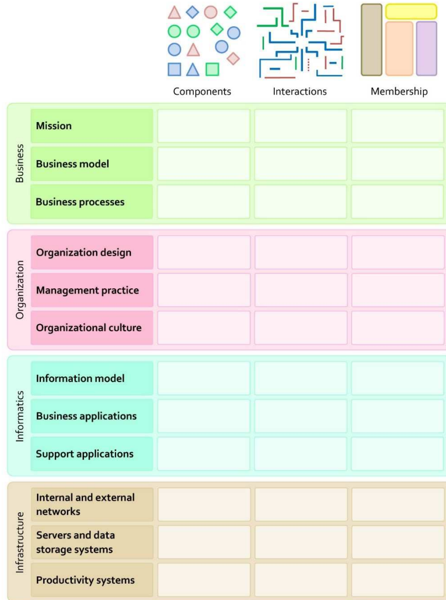
Fig. 3: A generic template for creating an enterprise architecture 'landscape' or 'blueprint.' A particular organizational element (such as a specific business process or IT system) is chosen as the focus, and its relationship to the building blocks and domains is analyzed via the component, interaction, and membership views. Depending on the element chosen, some (less relevant) fields may be omitted or considered only generally, while (more relevant) others will be expanded into detailed sub-diagrams.
