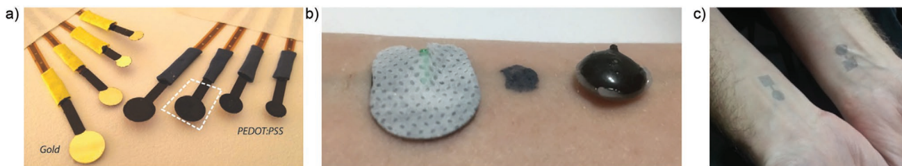
Figure 16. Three different approaches for conjugated polymer-based skin interfaces. a) PEDOT:PSS coated electrodes. Reproduced with permission. [242] Copyright 2014, Wiley-VCH. b) On skin light-cured PEDOT:PSS electrodes. Adapted under the terms of CC-BY 4.0 license. [240] Copyright 2018, The Authors, published by Springer Nature. c) Tattoo-style PEDOT:PSS electrodes, using temporary transfer paper. Adapted with permission. [42] Copyright 2018, IOP Publishing.
