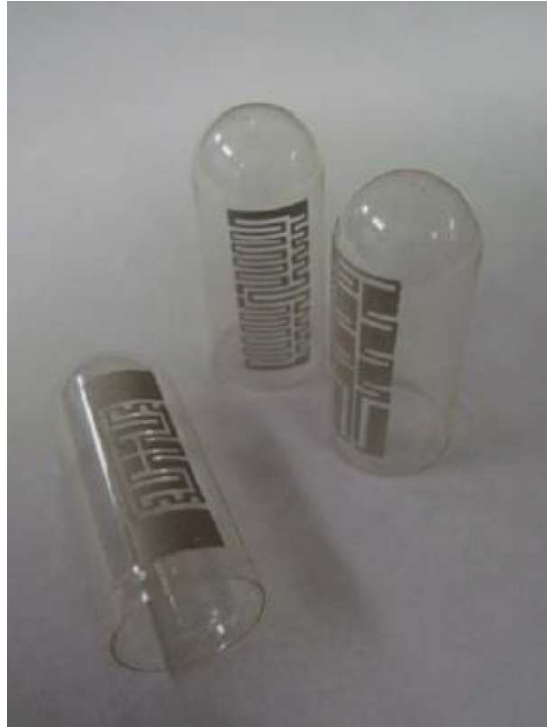
Figure 3.3: Bio-compatible capsule with embedded antenna (reproduced from [26])
