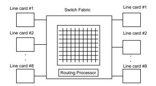
Fig. 5. Basic Data Plane Router Components.
