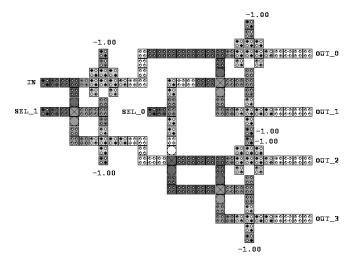
Fig. 8. Demux 1-to-4 implementation using QCA cells.
