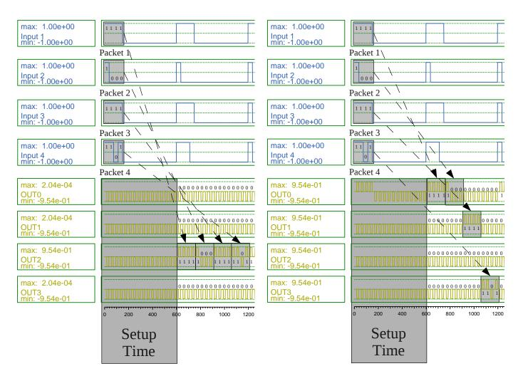
Fig. 14. Router results for first test where all packets are sent to output line 2.
