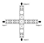
Fig. 7. Two wires crossing using multiple layers.
