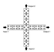
Fig. 6. Two wires crossing in a plane.
