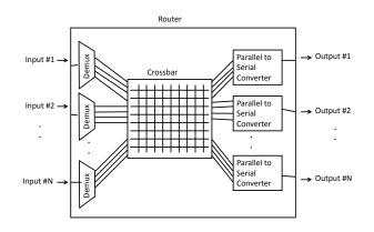
Fig. 10. Proposed Router Architecture.
