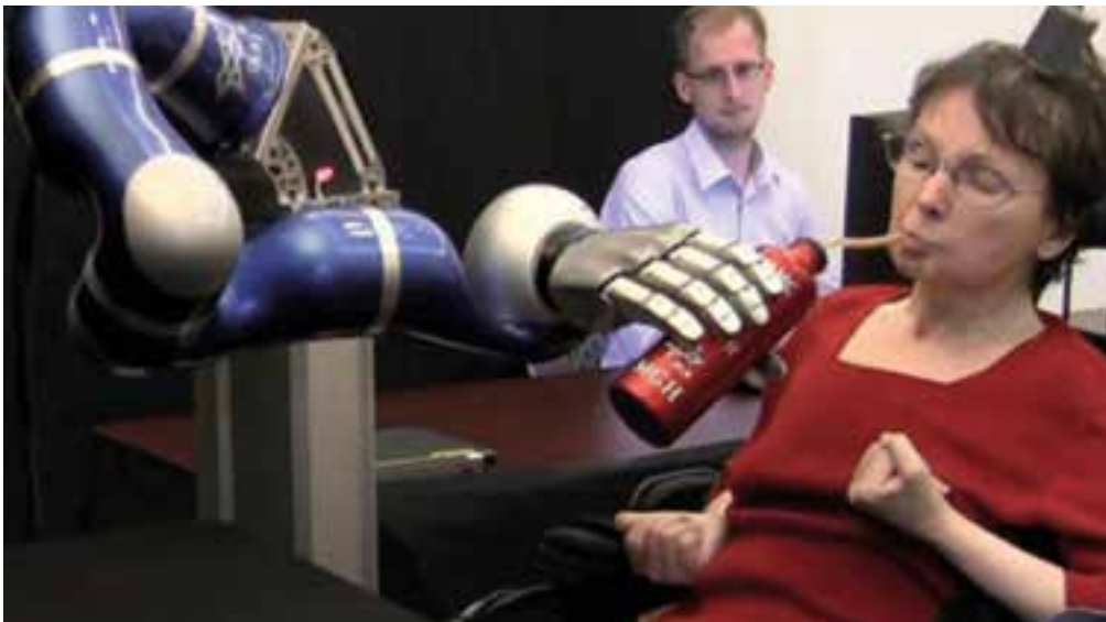
Left: A clinical trial of the cortical implant 'BrainGate' demonstrates how a person with paralysis is able to control a robotic arm using just their thoughts. © Brown University.
