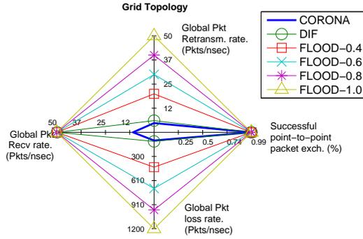
Figure 5: Radar plot for the setup of Fig. 4, presenting the successful packet transmission ratio, as well as the global packet send/receive/loss rate.
