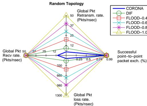
Figure 7: Radar plot for the setup of Fig. 6, presenting the successful packet transmission ratio, as well as the global packet send/receive/loss rate.
