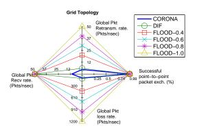
Figure 5: Radar plot for the setup of Fig. 4, presenting the successful packet transmission ratio, as well as the global packet send/receive/loss rate.
