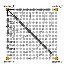
Figure 1: Coordination system setup. Each userselected vertex anchor broadcasts a single setup packet. Each node retransmits and updates its distance from the corresponding anchor, measured in hops traversed.
