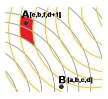
Figure 3: Using facing anchor points for packet routing may disallow the communication between certain network areas.
