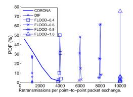
Figure 4: Probability distribution function (PDF) of nodes involved in the transmission of a packet from a random source to a random destination. A grid topology is used.
