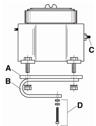
3. The hardened set screw and nuts (**D**) are used to tighten the switch to an I-Beam or cross member such as a Sampson post of an oil well pump jack.
