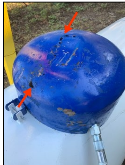
Protective cap deterioration observed.
