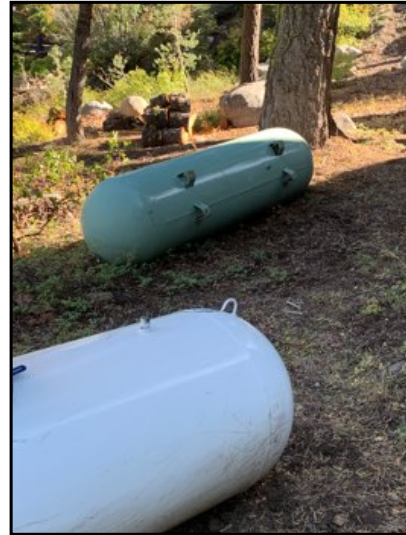
Recommend removal or proper storage of propane tank not in use.
