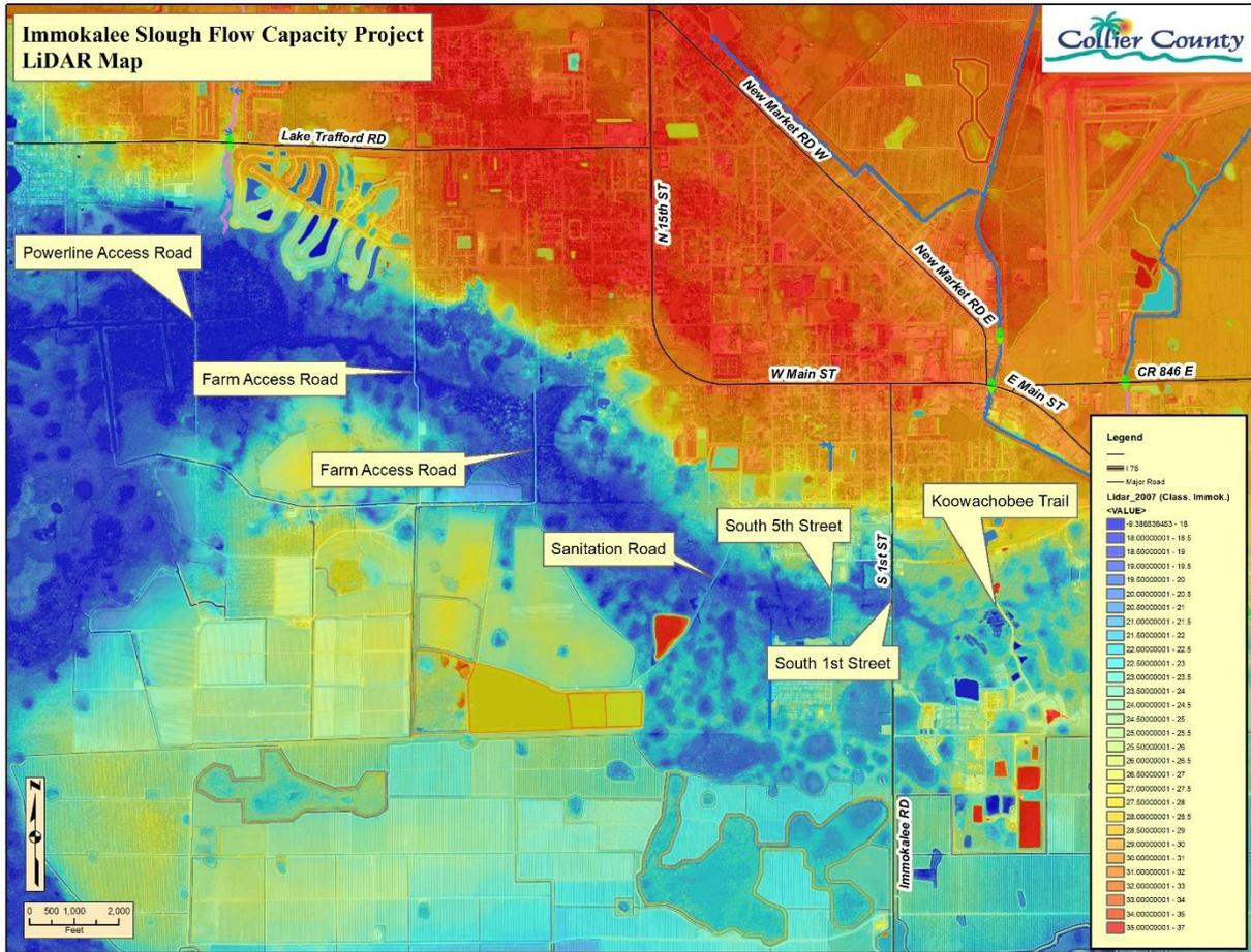
Water level staff gauges were installed at Sanitation Road and South 1<sup>st</sup> Street to be used as a comparison to staff gauge readings of the Lake Trafford water level. Water level readings from August 2016 to August 2017 showed the following approximate water surface elevation differences:
