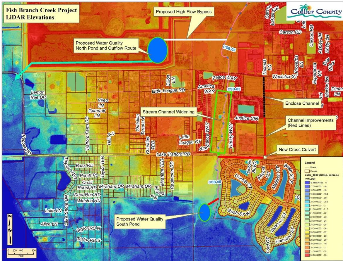
The ImmSIP modifications to the original Lochner Fish Creek conceptual project provide increased flexibility in selecting the order and timing of future stormwater facilities construction.
