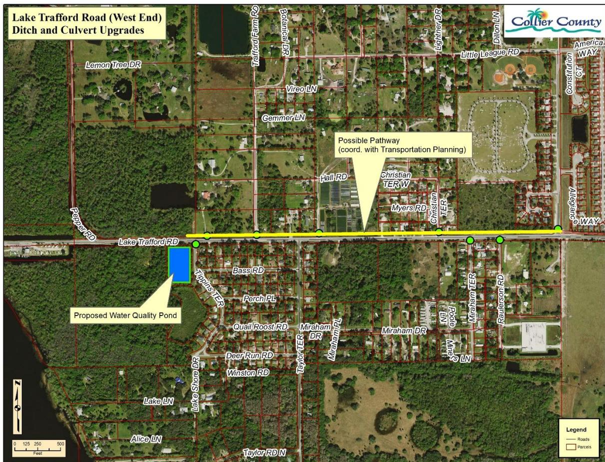
To construct the pathway, the existing ditch along the north side of Lake Trafford Road would have to be relocated northward. This would result in negative impacts to existing properties and wetlands. To accommodate the joint needs, the ImmSIP project proposes to enclose the existing ditch with a storm drain pipe sufficiently sized to provide the needed
