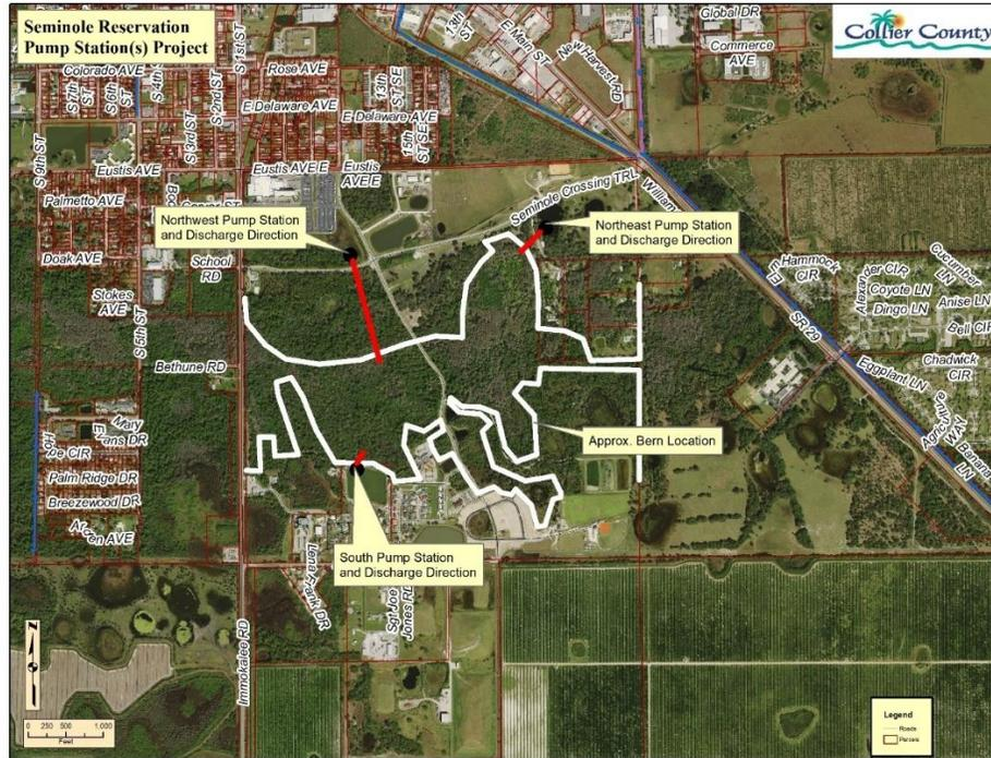
The proposed berm location is very rough in approximating potential development lands within the reservation. Additionally, the shown berm location could be the stormwater containment berms around new development areas and constructed at a sufficient elevation to serve a dual purpose. As shown on the following LiDAR elevation map, the berm location minimizes impacts on the slough wetland areas and storage capacity.
