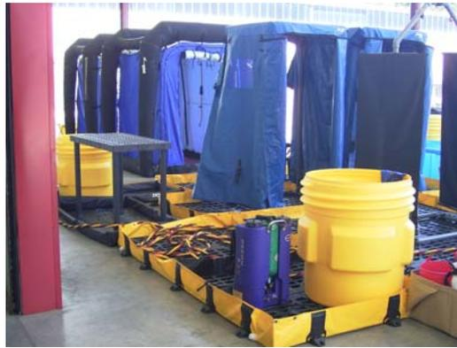
**FIGURE C-3 Yellow Containment Barrel and Diver's Umbilical with Berm and DECON Deck Grating**
