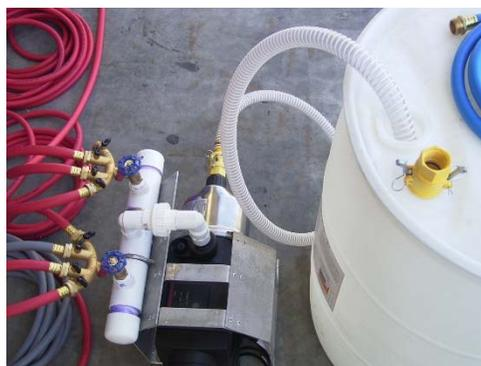
**FIGURE C-8 110V Electric Water Supply Pump with manifold, shut-off valves, with suction hose and red supply hoses to showers. White 50 gal clean water supply container**
