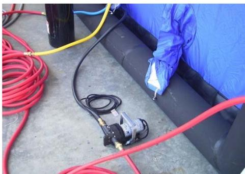
**FIGURE C-12 Zumro DECON Tent Dewatering 110V Electric Pump and Hoses**
