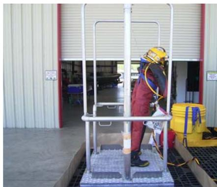
FIGURE C-2 4' X 9' X 9" Diver's Stage Berm with DECON Deck Grating
