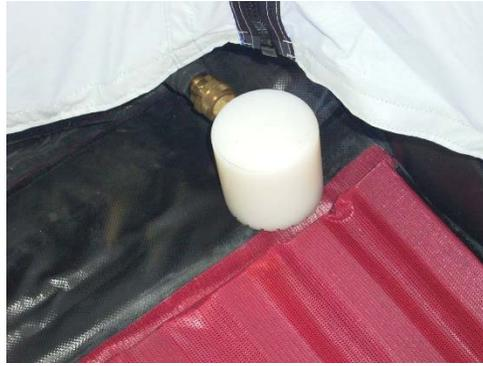
**FIGURE C-13 Zumro DECON Tent Dewatering Strainer (inside)**
