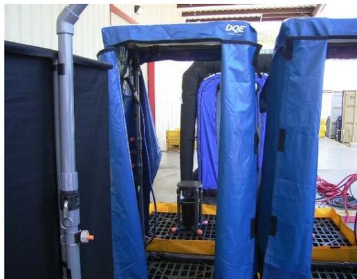
**FIGURE C-5 Rinse Showers with Yellow Berm and DECON Deck Grating**
