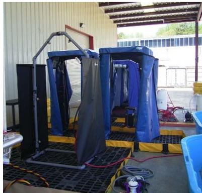
**FIGURE C-4 Wash Shower with Yellow Berm and DECON Deck Grating**
