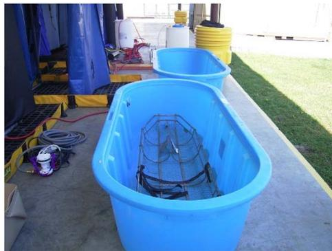
**FIGURE C-14 Emergency Wash Tub with Stokes Stretcher and Emergency Rinse Tub**
