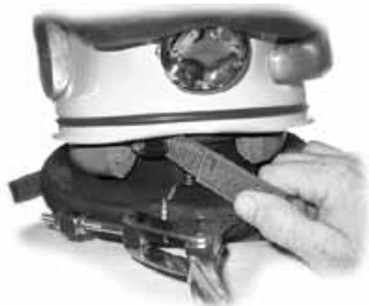
3. Place the Helmet over and onto the divers head and tighten the Chin Strap
