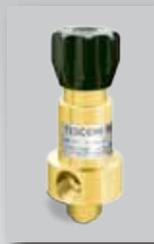
TESCOM 44-1300 Series is a high pressure, high flow (Cv=0.8 & 2.0) pressure reducing regulator that offers self-venting and balance valve design. Ideal for breathing air and special gas mix regulation for habitats or diving bells, typically integrated into a control panel.
