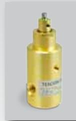
TESCOM 44-4000 Series is a dome loaded, spring biased regulator designed for pressure tracking application to maintain a constant differential pressure. Ideal for emergency backup breathing air and fire suppression systems, typically located outside the habitat or bell.
