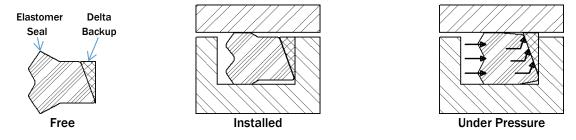
Typical Applications: Hydraulic Jars; High Performance Shock Absorbers - Cars/Trucks, Bicycles, Motorcycles, ATVs/UTVs, Snowmobiles; Oil & Gas High-Pressure Downhole Tools; Chemical/Fluid Metering and Injection Equipment; Valve Stem Seals; and any Low-Profile Dynamic/Oscillating Applications
