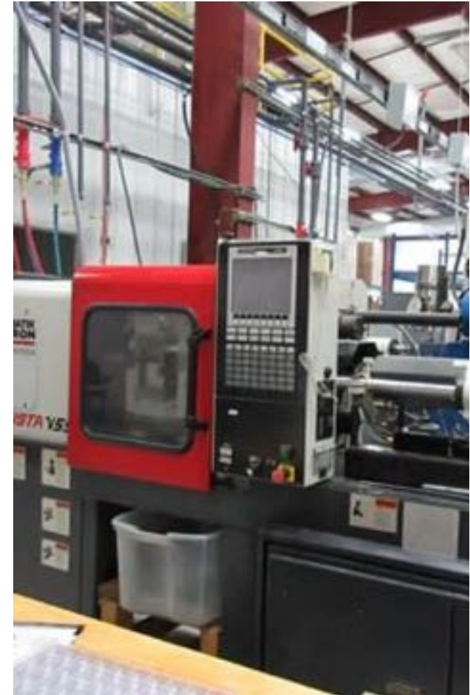
Upgraded injection moulding lines from Milacron ensure tight tolerances of moulded parts and reduce defects. ▲
